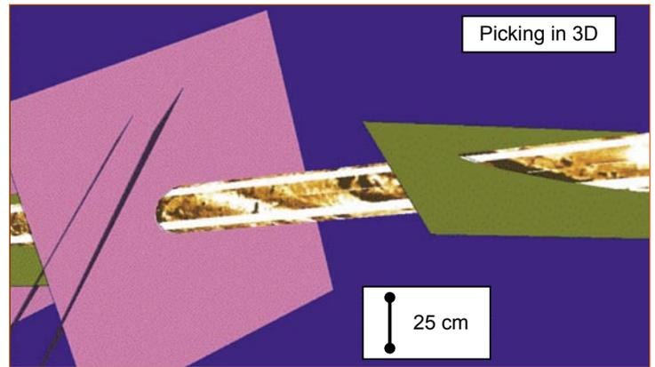
Figure 6: Interactive BHI interpretation in 3D. A utility to pick features in 3D has been developed to interpret high level feature based on both BHI and seismic data.
