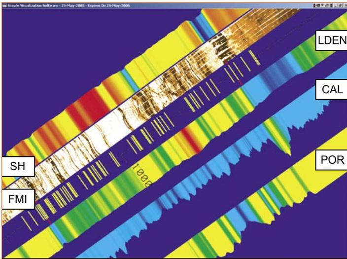
Figure 3: Combination of BHI images, BHI picks and open logs in 3D (zoom of Figure 2). The fractures are represented by simple lines perpendicular to the well trajectory to help the analysis of the fracture/BHI/open-hole log relations.
