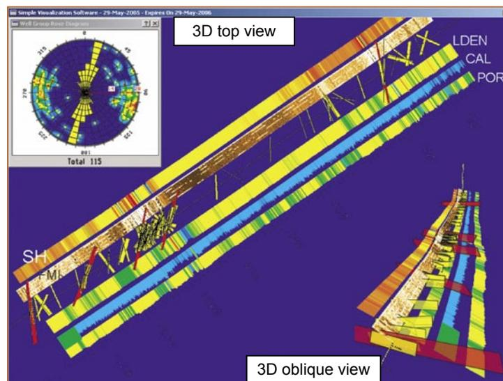
Figure 2: Combination of FMI images, fracture interpretation and open logs in 3D. The fractures displayed correspond to electrically conductive fractures of different width. Minor and major fractures are represented by the yellow and red rectangles respectively, with true dip and strike. The rose diagram of the fractures is shown in top left corner with the density of poles to the fracture plane as a property.
