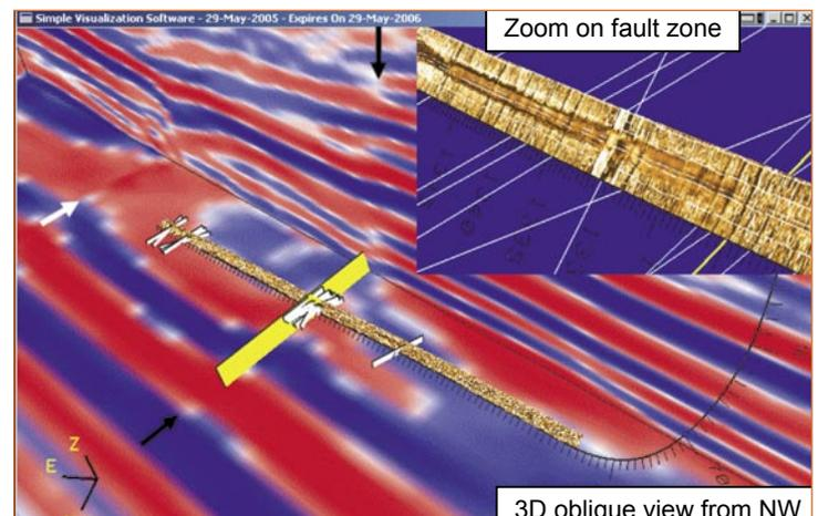
Figure 4: Combination of seismic data with BHI. The displays correspond to a chair display showing one cross section in the back and a time slice immediately below the well trajectory. The presence of a fault (indicated by the black arrows) is highlighted by the fracture cluster (white and yellow rectangles) interpreted on the BHI.
