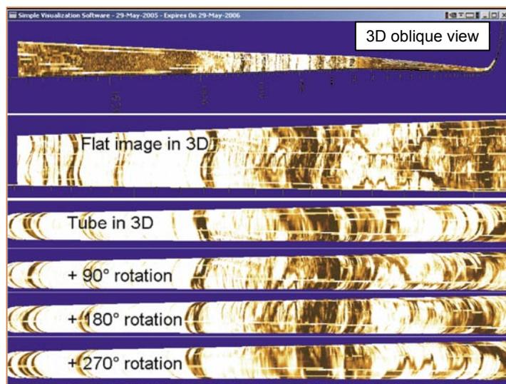
Figure 1: BHI picture displayed in SVS as flat picture (top 2 images) or around a cylinder (bottom 4 images).
