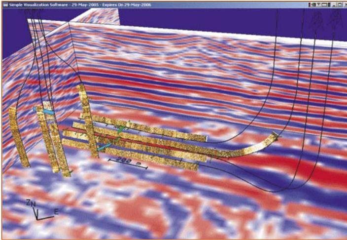
Figure 5: Combination of seismic data with BHI. The display corresponds to a chair display showing 2 perpendicular cross sections and time slice immediately below the well trajectories. The rectangles correspond to electrically conductive fractures picked on the BHI. Loading multiple wells enables the interpreter to assess the possible extension of features in nearby wells. For example, this is particularly useful when attempting to identify fracture corridors in the subsurface.
